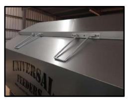
**STEP 77:** Attach the lid handles to the lid using holes provided in the lid.
