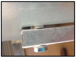
**STEP 46:** Attach lid hinge to end, one washer between bolt and RHS, three washers between RHS and end.
