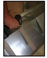
**STEP 24:** Fit the seven straps to base. Holes located at the top of the bend of the base.
