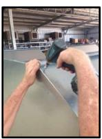
**STEP 67:** Place one screw up top of side connecting to end.
