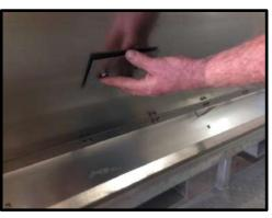
**STEP 38:** Attach supports to divider. Plate is to go onto the outside.
