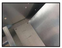
STEP 12: Fit base to ends. Line up holes.
