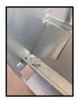
**STEP 25:** Adjuster bracket (Left and right).
