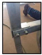
**STEP 3:** Loosely tighten nuts to allow some movement in post.
