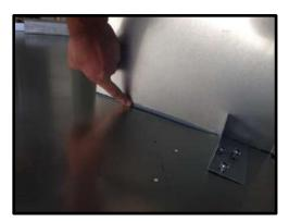
**STEP 27:** Selastic gap between the base and the end (Do not selastic below adjuster bracket). Tighten.
