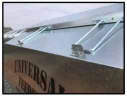
**STEP 78:** Tek screw angle into holes provided. This will form self-locking of lid.
