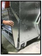
**STEP 75:** Place rain guards on all 4 corners of feeder (There is left and right).
