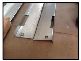
**STEP 49:** Attach cage nuts to upper adjusters. One each end (Note which way the cage nut is attached).
