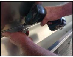
**STEP 34:** Attaching straps to bottom of dividers.
