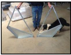
**STEP 45:** Always remember there is a left and a right side, so fit lid ends alternatively to lid RHS hinge.
