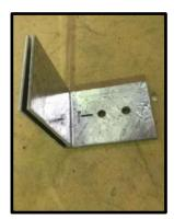
**STEP 19:** Place angle with 'T' on top of the other angle. This will form a gap which the upper adjuster will go between.
