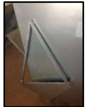
STEP 45: Tighten so lid hinge is firm but moves freely.
