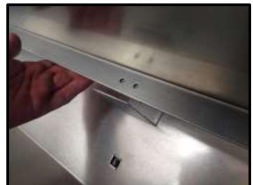
STEP 30: Attach straps that are screwed into base to divider. Holes are to be lined up.
