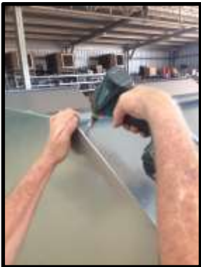
STEP 64: Place one screw up top of side connecting to end.
