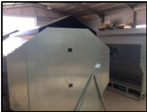
STEP 67: Place lid onto feeder.
