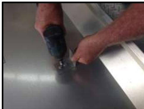
STEP 20: The two holes in the base are for the angle piece.
