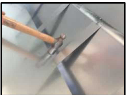
STEP 34: If divider needs straightening so straps line up, always hammer on corners.
