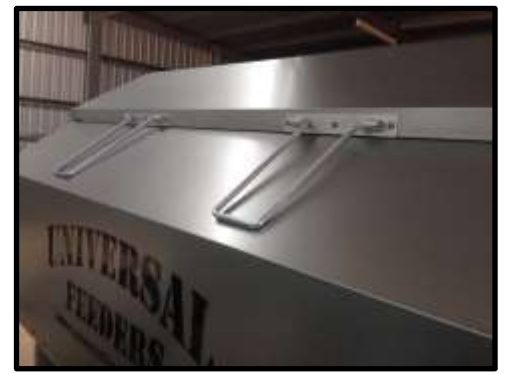
STEP 72: Attach the lid handles to the lid using holes provided in the lid.
