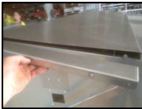
STEP 83: Place bridging piece under lid.
