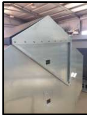
STEP 68: Connect lid hinge to feeder.
