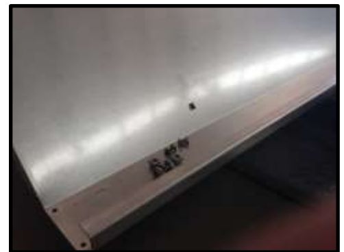
STEP 6: Diagram of cage nuts.
