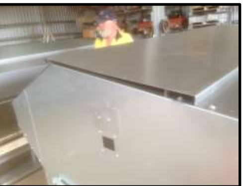
STEP 82: Place lid onto feeder.
