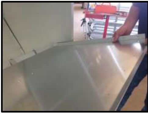
STEP 25: Slide dividers through slot in end.
