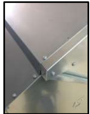
STEP 69: Connect lid hinge to feeder.
