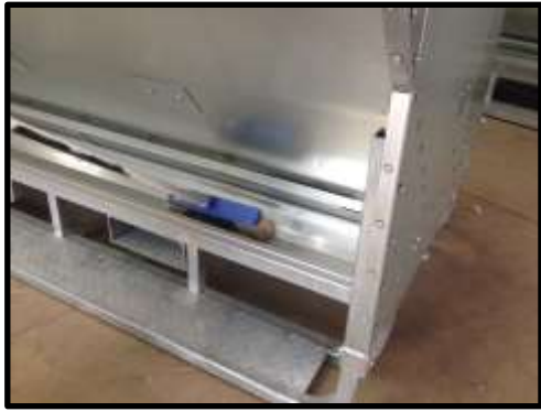
STEP 73: Sweep the base and all areas of feeder of steel filings.
