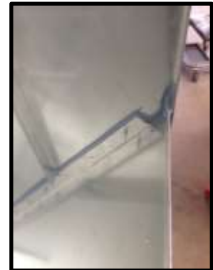
STEP 57: Silicon the divider to the end.
