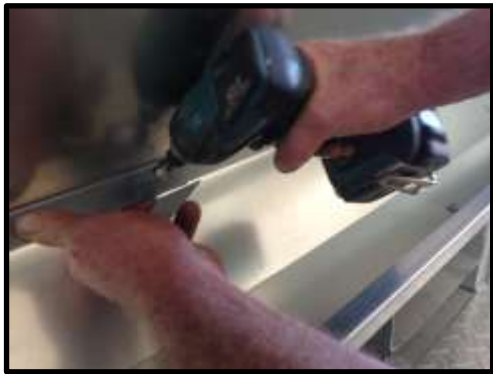
STEP 31: Attaching straps to bottom of dividers.
