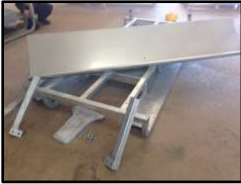
STEP 1: Lay posts out on each corner (Left and right) and base onto frame and lid hinges.
