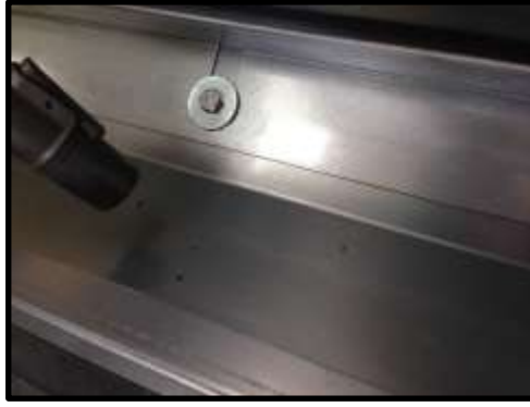
STEP 74: Ensure completely clean as any filings left will rust.
