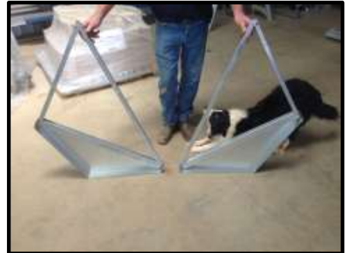
STEP 42: Always remember there is a left and a right side, so fit lid ends alternatively to lid RHS hinge.
