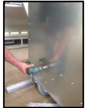
STEP 27: Tek screw to end.
