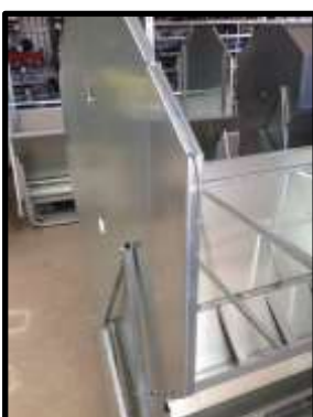
STEP 58: Silicon the end extension ready for sides..
