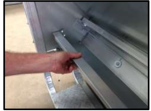
STEP 51: If attaching ad-lib pieces line up with the two holes on the ends.
