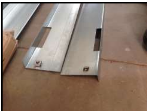
STEP 46: Attach cage nuts to upper adjusters. One each end (Note which way the cage nut is attached).
