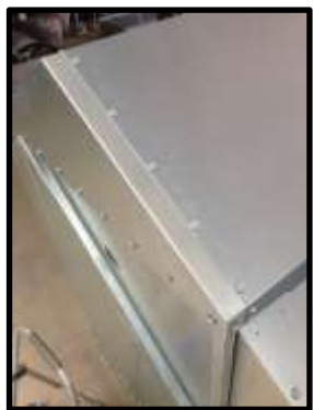
STEP 71: Ensure all screws are fitted to holes.
