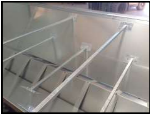
STEP 37: Finished look of Large and Extra-large feeders (Medium has only one top support).
