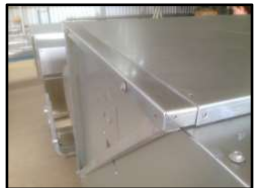
STEP 84: Fully tek screwed. Top tek screws must be the shorter screws. Side screws longer tek screws. Attach the 2 lid handles in the holes provided in lid.
