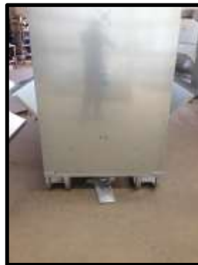
STEP 29: Both dividers in place. Ensure all holes fitted with tek screws.
