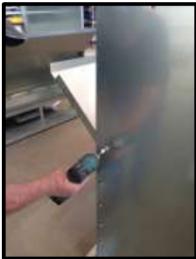
STEP 28: Attaching divider to end.
